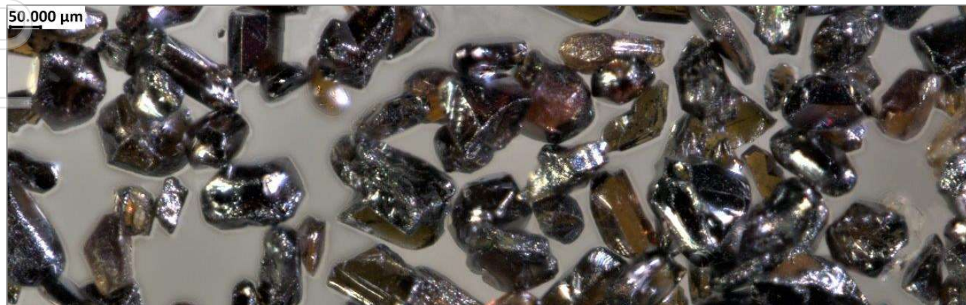
Figure 8: Photomicrograph of high purity rutile product 97.2% TiO 2
