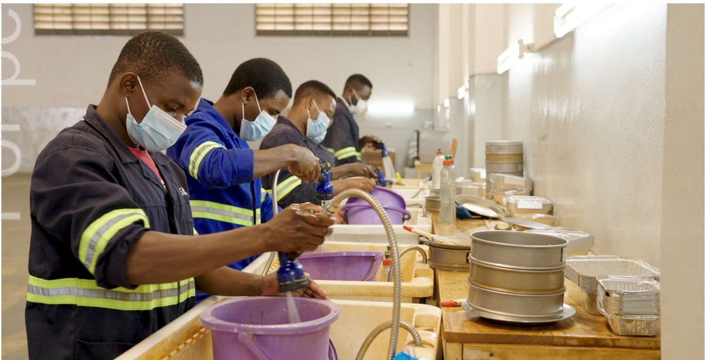
Figure 2: Sample de-sliming at the Company's laboratory facility in Malawi
